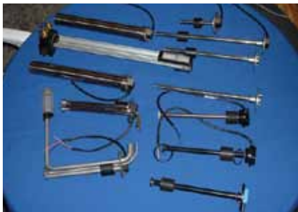
Top: Typical aluminum tanks for powerboats. Above: A selection of tank senders from Wema.
