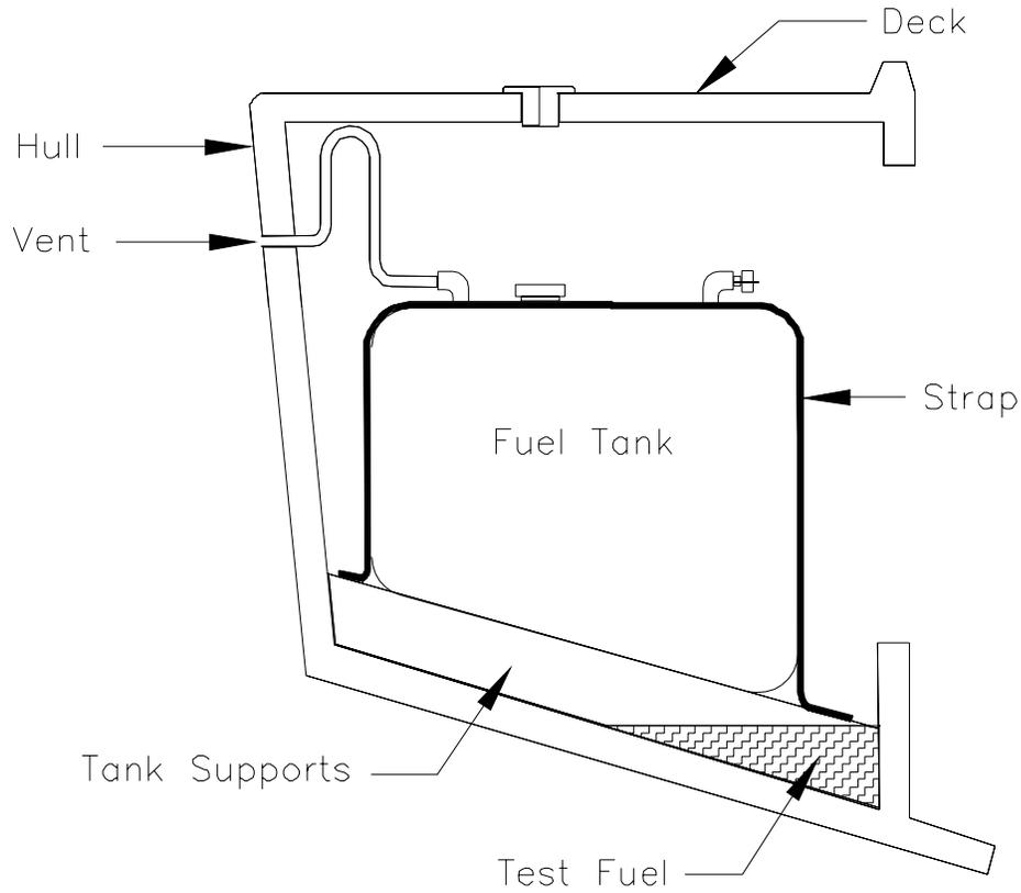
FIGURE 2 - ENCLOSURE - ABOVE DECK INSTALLATION
