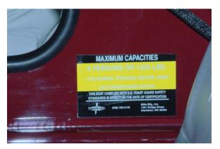
Recreational boat manufacturers are required to put a capacity label on mono-hull boats under 20 feet in length. See 33 CFR Part 181 Subpart I - General. You will see a similar label on many other types of boats, including canoes, kayaks, pontoon boats and inflatables. The manufacturers voluntarily (in the USA) put these on other boats because it is good business and safety sense to do so. In Canada and Europe the label is required on all recreational boats (with a few exceptions).
